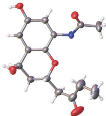
Fig. 2 The single-crystal X-ray structure of 1
